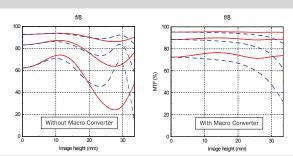
The following graph shows the effect on close range use for the H system wide angle lenses when using the Macro Converter H.
